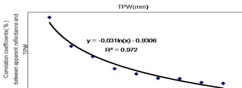
Figure4. negative and inverse correlation between apparent reflectance (%) and TPW (mm)
