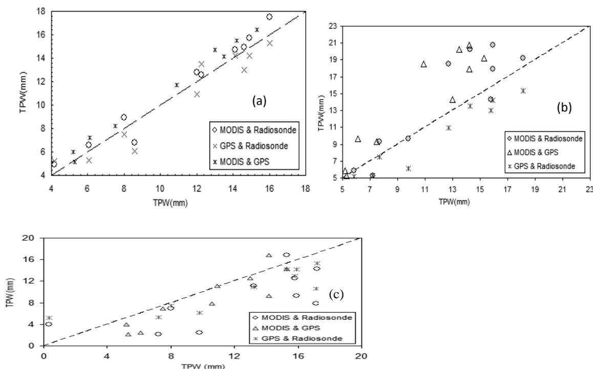
Figure3. The correlation between Radiosonde and Near-IR TPW for band ratios (a): 19 to 2, (b): 18 to 2 (c): 17 to 2.
